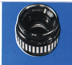
Meogon 5.6/80 mm Lens — Cat. No. 703 450 — Branch No. 392 812 110 302 has an asymmetrical optical construction and is composed of six elements in four groups. It is determined for advanced amateurs and photo laboratories and enables enlarging from 6×6 cm negatives. Its attaching thread is M39×1Sh4.
