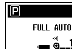
Example 2: Exposure-mode dial set to , full-auto mode. Top part of display has turned black.
