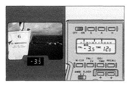
If another reading is made when the  $\square$  mark is displayed, the meter will indicate the difference in brightness between the calculated reading and the new reading. Refer to page  $36 \sim 38$  for more information.
