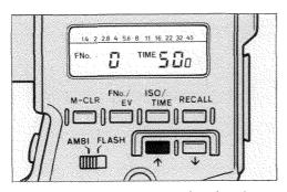
In ambient metering mode, the shutter speed can be set from 1/8000 sec. to 30 minutes, plus 1/50 sec. (which comes after the 30 min. when pressing the decrease key) for taking cine readings at 24 fps.
