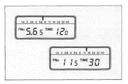
When taking ambient-light readings, changing the ISO or shutter-speed setting will change the f-number displayed.
