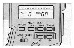
The Spotmeter F has two display/measurement modes, f-number (FNo.) and exposure value (EV). Press the FNo./EV key to display the desired mode on the external LCD display panel.
