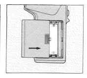
The Spotmeter F is powered by a single AA-size battery. A 1,5-volt alkalinemanganese or carbon-zinc battery or 1.2-volt 4. Replace the cover and slide it back into its nickel-cadmium battery can be used. To original position. install the battery:
