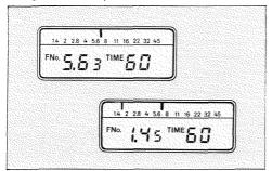
To use the Spotmeter F's memory function, take a reading and press the memory key. The display will go blank for a moment and then reappear after the reading is entered into the memory. You can now take a second reading which will be indicated by a pointer on the analog scale and by a new
