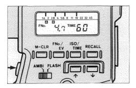
on the analog scale next to indicated the fnumber. A  $\square$  mark will also appear indicating that any further readings will be displayed as differences in brightness from the calculated reading. These readings will also be indicated by a fourth pointer on the analog scale. Refer to page 36  $\sim$  38 for more information.
