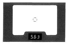
In addition to the meter's external display, there is also a digital display in the viewfinder that lets you to monitor the exposure information while taking a reading. The f-number, EV number, and brightness differences are displayed with tenth-stop accuracy. The measuring spot defines the meter's 1° angle of acceptance.
