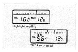
To make a highlight reading, first press the memory-clear key to clear any previously memorized readings, then proceed as follows:
