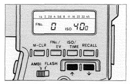
2. Press the increase key to set higher film speeds; press the decrease key to set lower film speeds. The setting changes by 1/3 stop each time either key is pressed and continuously when a key is held down. Any film speed from ISO 12 to ISO 6400 can be set.
