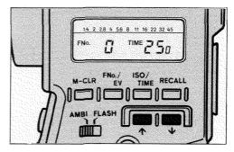
To change the shutter speed, press the increase or decrease key until the desired speed is displayed. Each time either key is pressed, the display will change by one full stop. The speed changes continuously when either key is held down.
