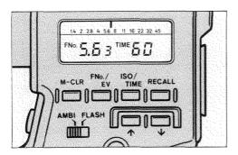
5. Set your camera to the shutter speed and aperture shown on the meter's digital display.
