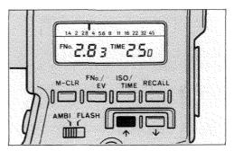
If desired, other aperture/shutter speed combinations can be displayed by pressing the increase or decrease keys.
