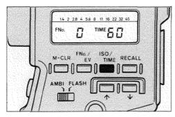
**3.** After setting the film speed, press the ISO/TIME key to return to the time-display mode.
