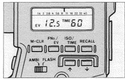
The EV display mode is useful for checking contrast ratios (p. 39), luminance (p. 40), and other lighting conditions. In this mode, the display readout will be in EV steps, and only changes in the ISO setting will affect the EV display.
