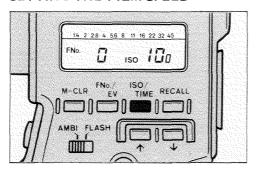
1. Press the ISO/TIME key to display the ISO film-speed setting. If the battery has just been installed, "100" (ISO 100) will be displayed.
