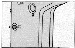
The viewfinder display can be illuminated for easier reading in low light by pressing the display illumination button located on the meter's grip.
