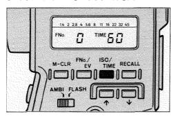
After setting the film speed, press the ISO/TIME key to put the meter in time-display mode. The display will show the most recently set shutter speed. If the battery has just been installed, "60" (1/60 sec.) will be displayed.
