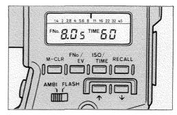
In f-number mode, a digital aperture figure will appear next to the "FNo." indication in the display panel. Next to this figure is a small one-place decimal display that shows the necessary exposure decrease in 1/10 stops. For example, if the aperture display is  $f/8.0_0$ , the lens should be set at exactly f/8. If the display shows  $f/8.0_5$ , then the exposure should be decreased by 5/10 (1/2) stop. The lens aperture should be set halfway between f/8 and f/11.
