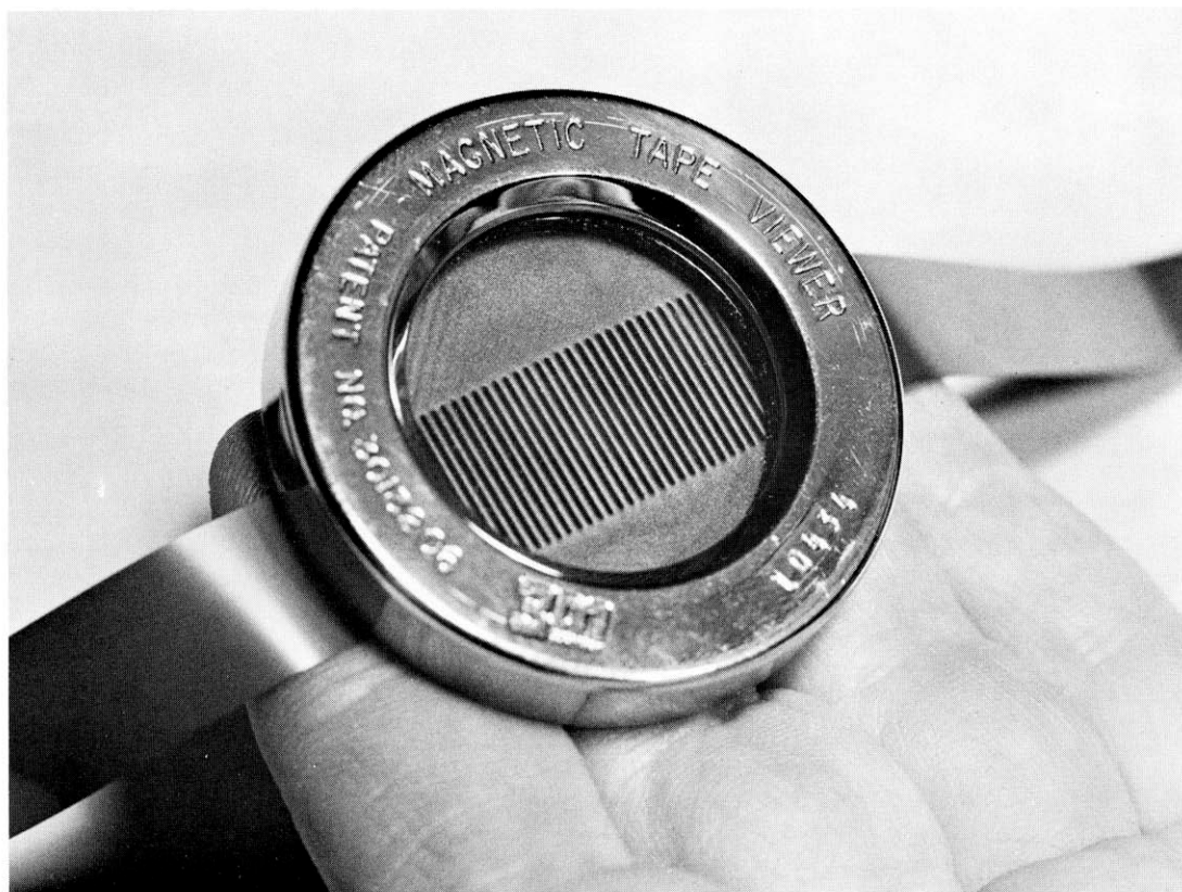
Magnetic pattern as seen with 3M viewer.
