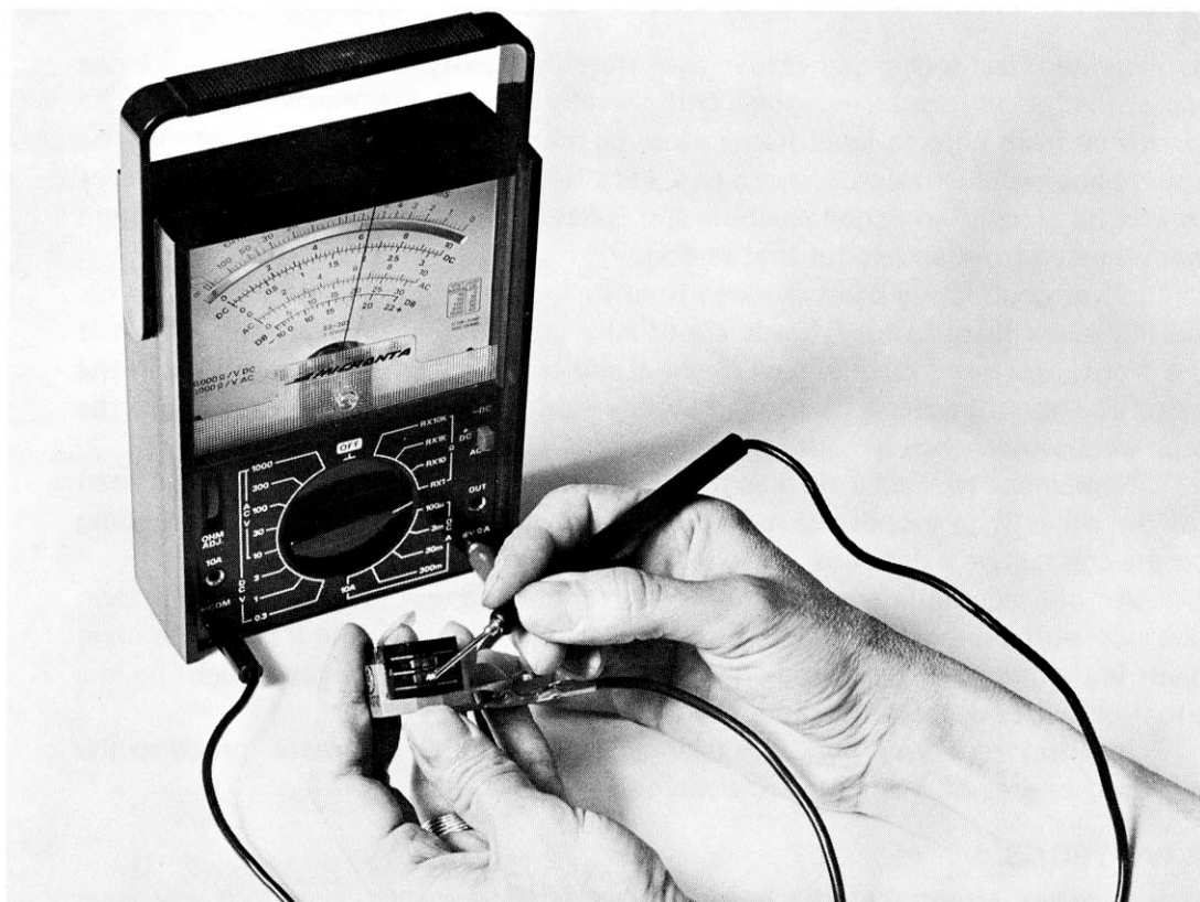
Checking for resistance between core and frame.
