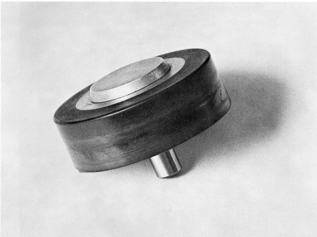
Figure H – Grooved capstan idler can cause steering with resulting skew
