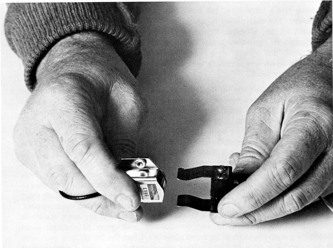
Induction loop jig is held in place by means of spring clips.
