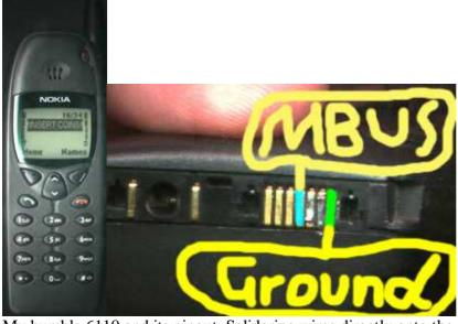
My humble 6110 and its pinout. Solidering wires directly onto the phone does not hurt it if you were wondering. Since people have asked I have put more connection pinouts at the bottom of this page, 8810,3310,3210, 8210, 8250
