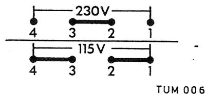
Fig. 2 Connections for two voltage ranges
