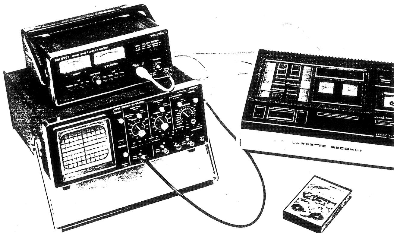
Fig. 6 Wow and flutter measurements of a cassette recorder
