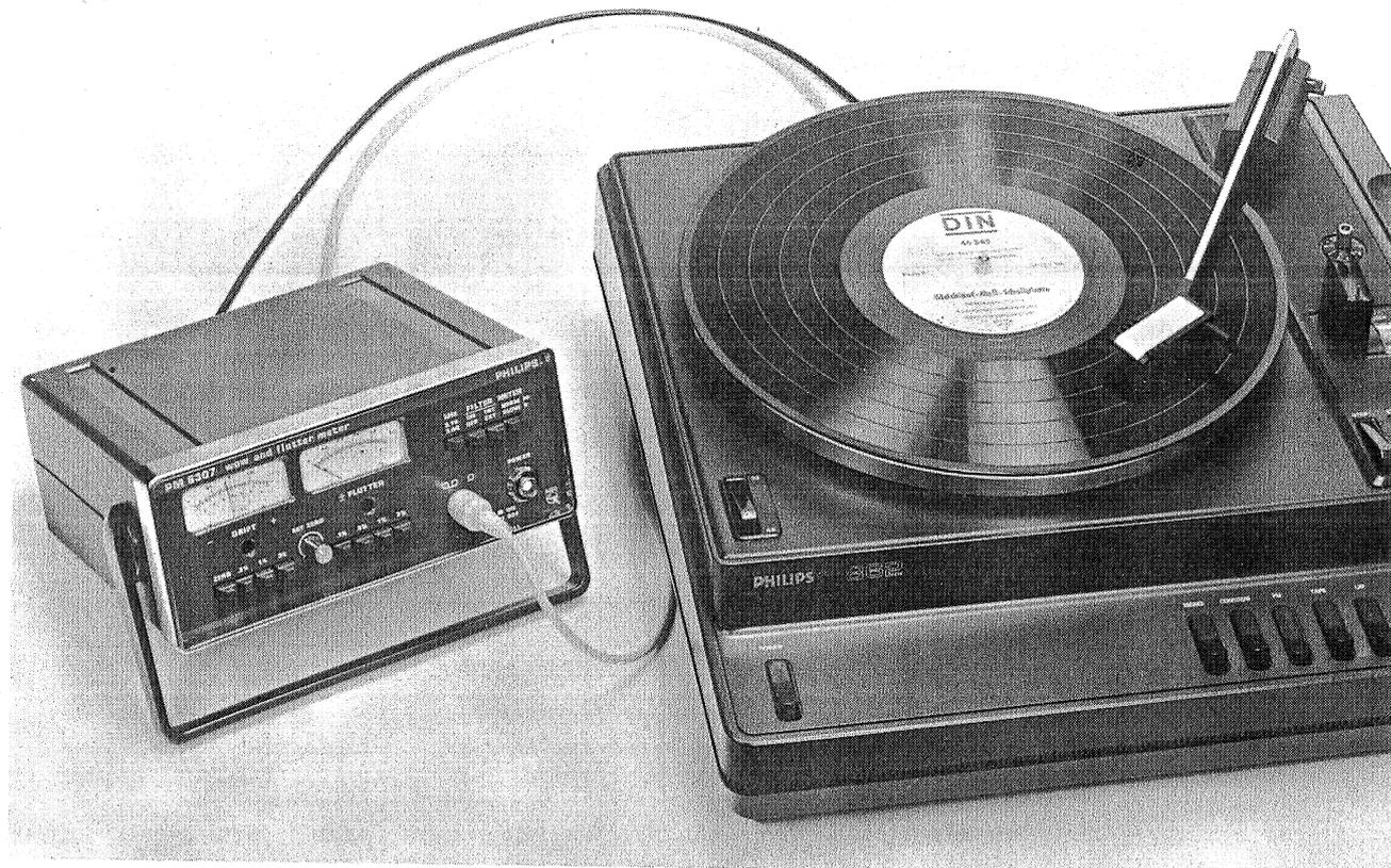
Fig. 5 Wow and flutter measurements of a record player
