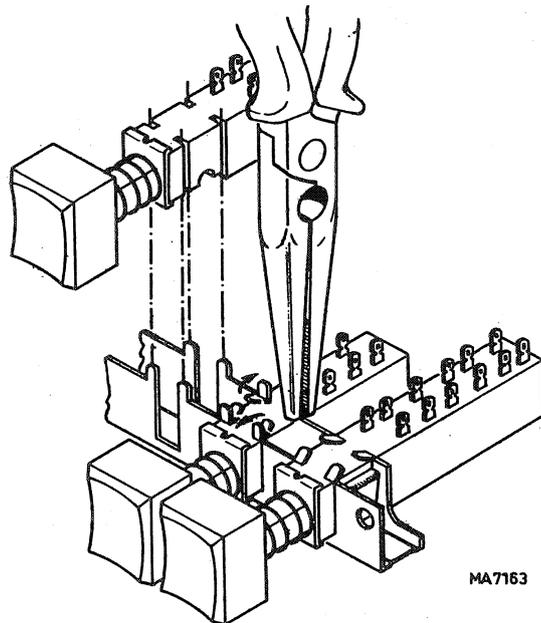
Fig. 8 Replacing a switch of the pushbutton unit
