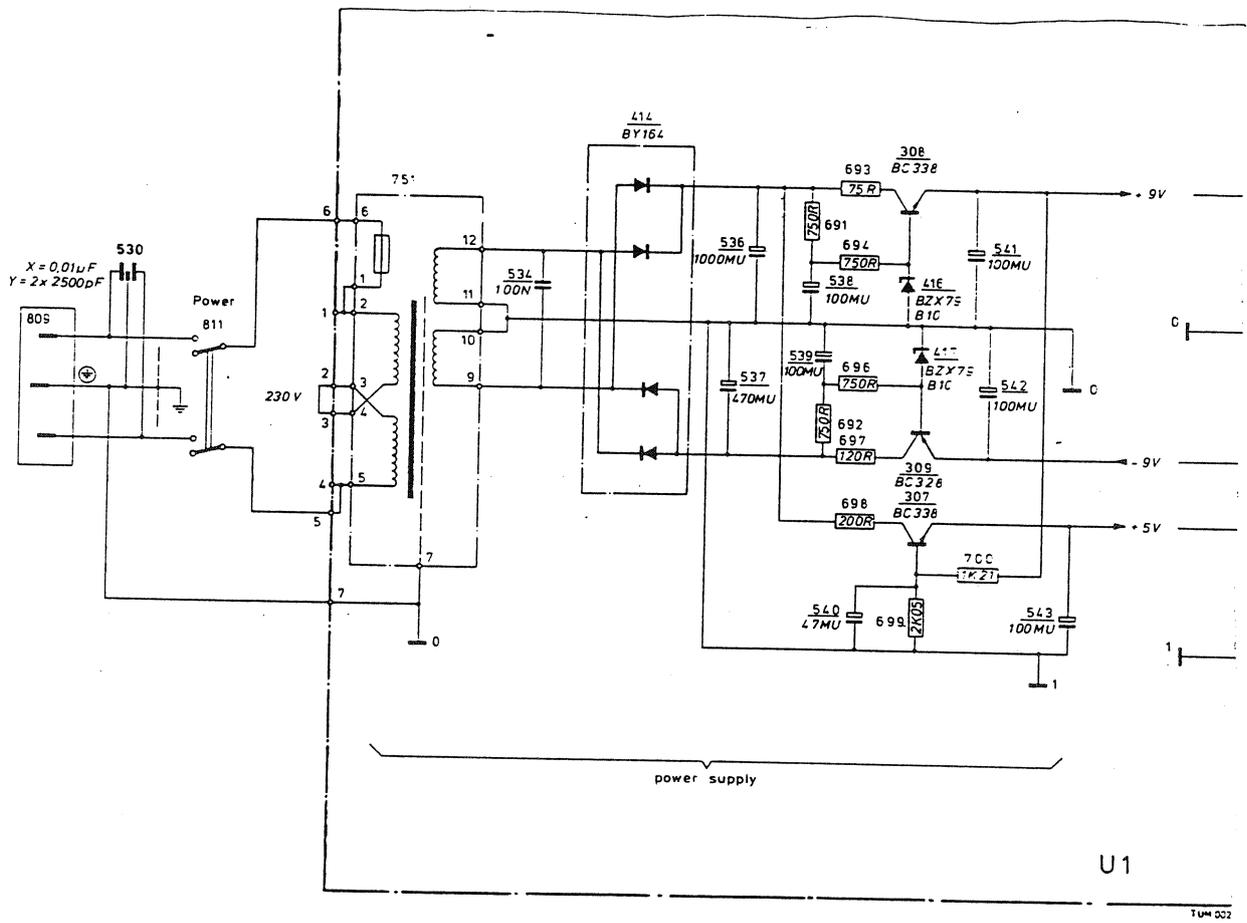
Fig. 15 Circuit diagram of power supply PM 6307
