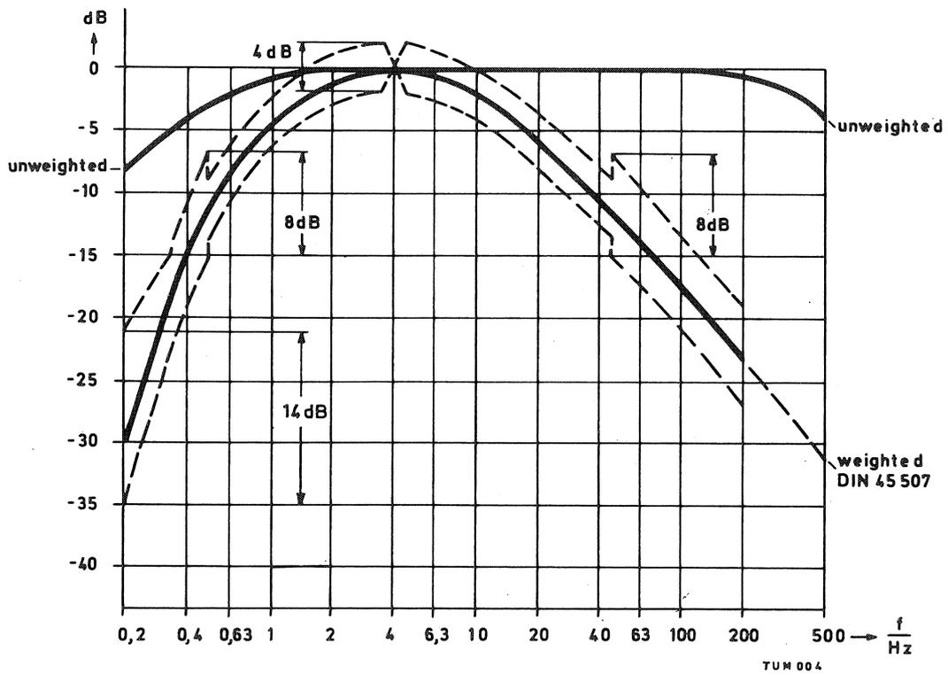
Fig. 7 Transmission characteristic of evaluated and non-evaluated measurements
