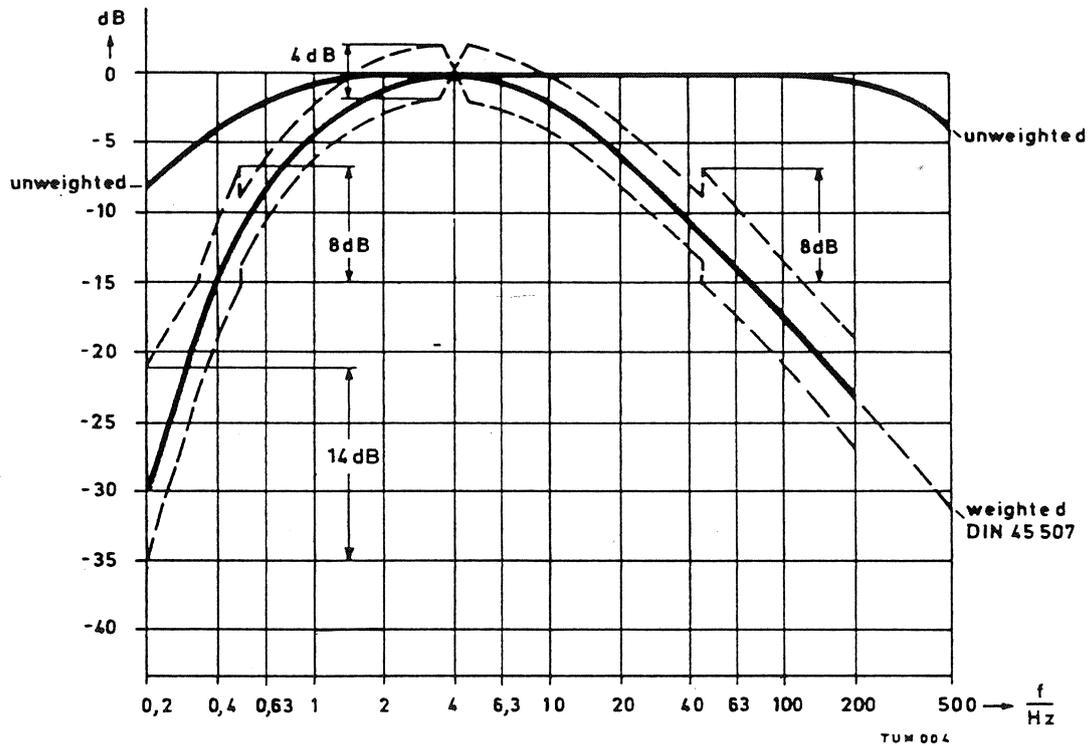
Fig. 7 Transmission characteristic of weighted and unweighted measurement
