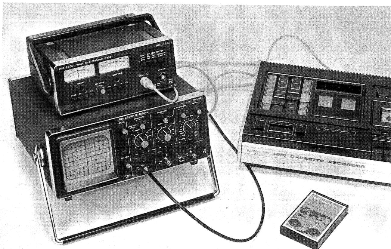
Fig. 6 Wow and flutter measurements of a cassette recorder
