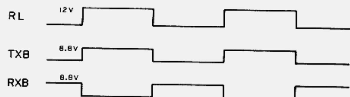
Fig. 10 STANDBY keying timing chart
