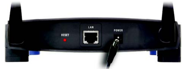
Figure 4-2: Connect the Power
