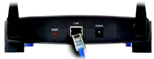
Figure 4-1: Connect the Ethernet Network Cable
