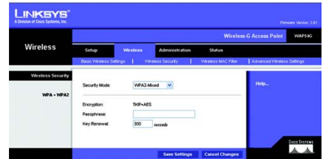
Figure 6-15: Wireless Security - WPA2-Mixed Screen
