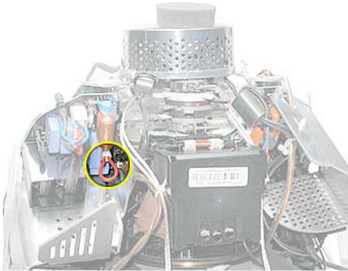
Voltage Jumper Location
