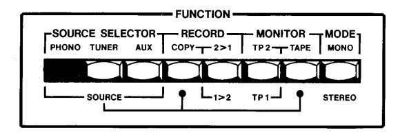
Referring to the first FUNCTION switch drawing, above, let's look at the signal flow from left to right. The SOURCE SELECTOR group consists of three interlocking buttons, of which only one is pushed in at a time. The diagram above shows that the PHONO stage has been selected as the program source in this case. As shown in the diagram, below the SOURCE SELECTOR, RECORD and MONITOR groups, the selected SOURCE material is fed to both the RECORD switch pair and the MONITOR switch pair.
