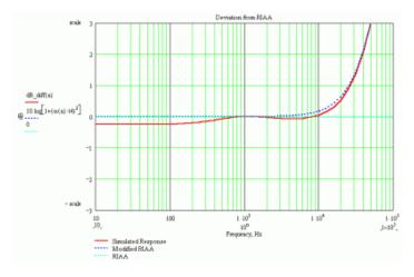
As seen in the graph, the Allen Wright modification boosts the treble by 0.5 dB at 20 kHz, a modest change by any measure. The VSPS follows this modified response.
