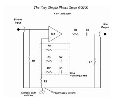
The circuit is so basic that each component can be discussed individually. I've split the design into low impedance (Lo-Z) and high impedance (Hi-Z) versions. The Lo-Z circuit is a low noise version optimized for Grado and other low inductance cartridges (<300 mH), the Hi-Z version is better suited for "traditional" MM cartridges with high inductance (>300 mH). The performance difference is small, both varients will work fine with any source.
