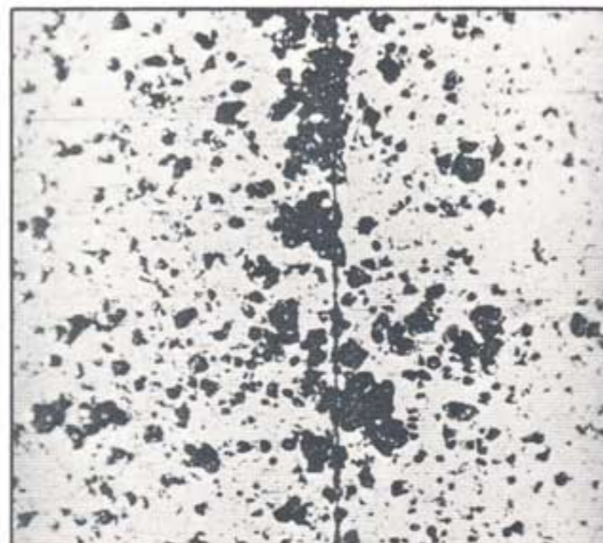
Gap environs of Crystal Ferrite Head. Gap environs of poly ferrite head.
