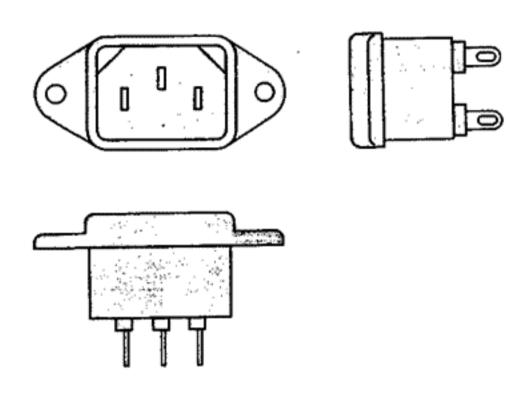
AC INLET to be installed on machines
